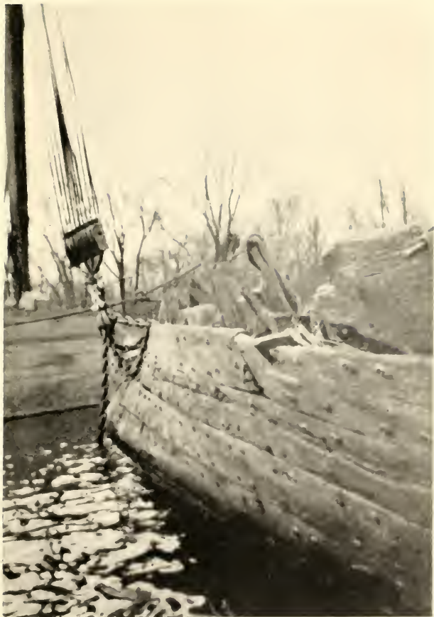
STARBOARD QUARTER OF THE "NIAGARA" : NOTE THE WARTY APPEARANCE OF HER PLANKING WHERE THE ACID OF THE SPIKES HAS PRESERVED THE OAK
